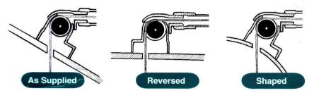
Adjust location if necessary to avoid any obstacles on the tank such as pipework, bulges, overflow outlet, etc., and trace its outline on the tank roof. Check that the Guide Pipe, when fitted into the Main Pulley Housing, will be at least 10mm (3/8") clear of the tank wall.
